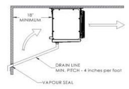
Proper air flow through the coil is very crucial to unit performance and maintenance of design storage space temperature. Therefore, a minimum of 18 inch space must be provided behind the unit for unrestricted air flow through coil.
